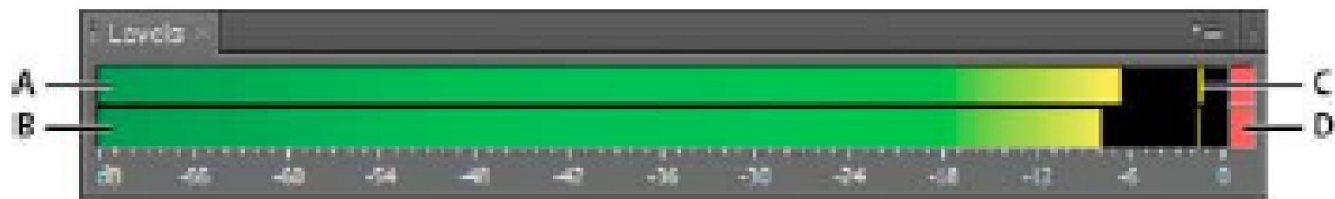
A Left channel B Right channel C Peak indicators D Clip indicators
