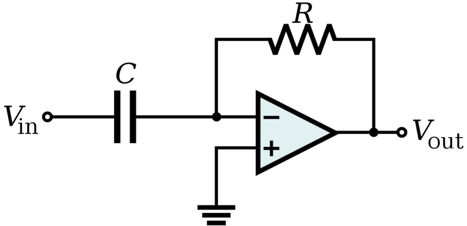
$$V_{out} = -RC \frac{dV_{in}}{dt}$$
