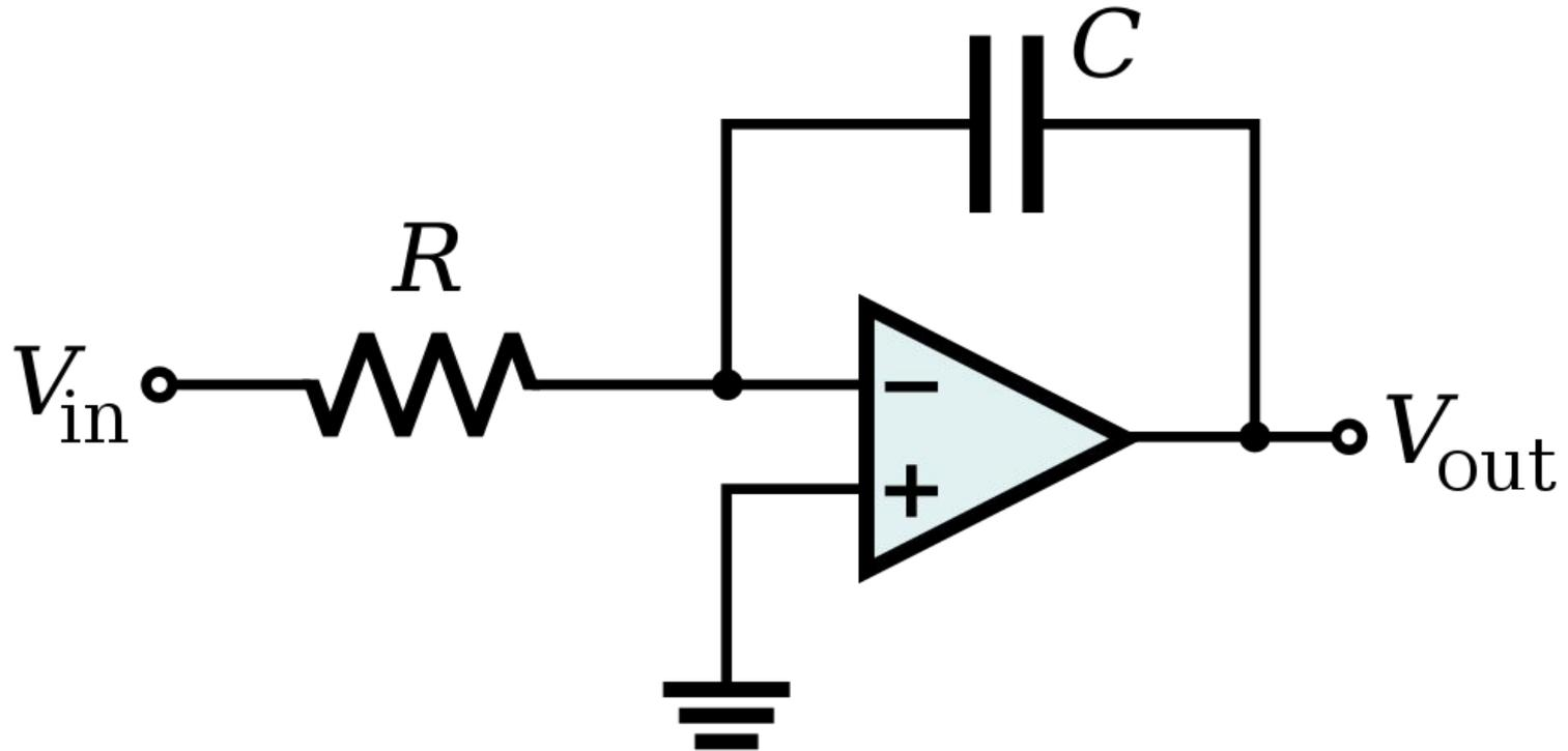
$$V_{out} = - \int_0^t \frac{V_{in}}{RC} dt + V_{initial}$$
