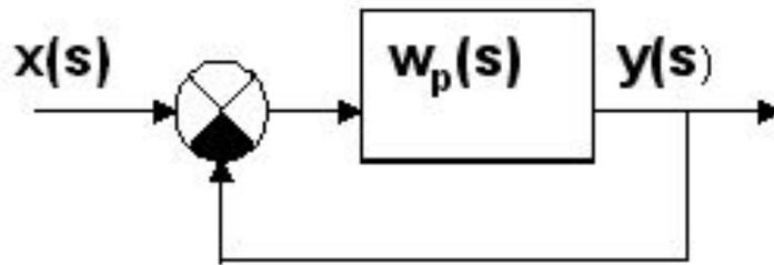
$$w_p(s) = \frac{K}{(T_1S + 1)(T_2S + 1)(T_3S + 1)} = \frac{K}{D(s)}$$
