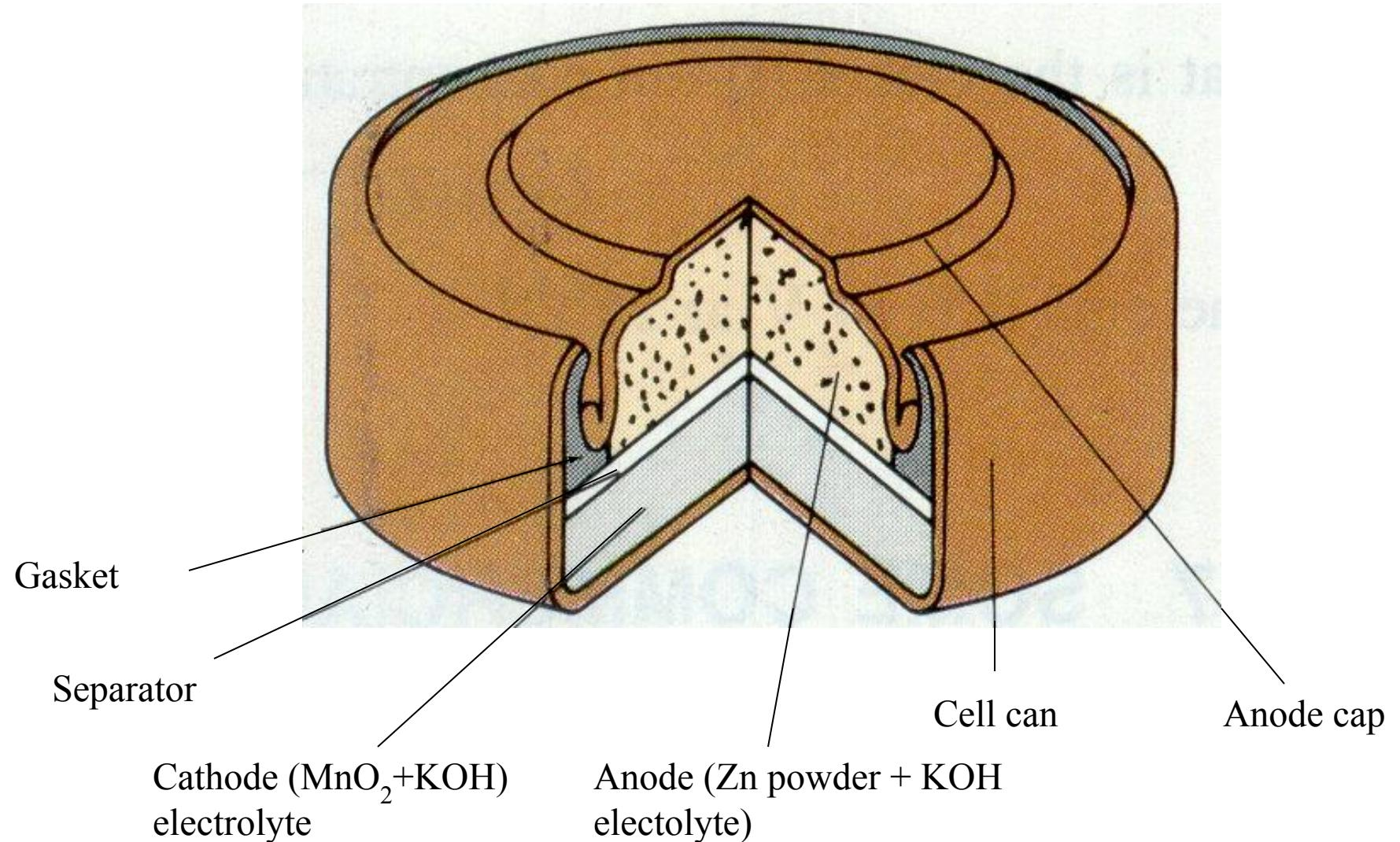
**A small alkaline dry cell.** The anode is zinc powder and the cathode is  $\text{MnO}_2$ , as in the Leclanche cell; however, the electrolyte is KOH.
