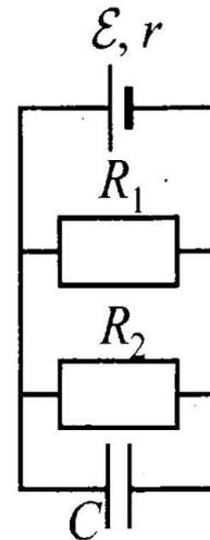
$$u_c = \frac{\varepsilon}{\frac{R_1 R_2}{R_1 + R_2} + r} * \frac{R_1 R_2}{R_1 + R_2} = \frac{\varepsilon(R_1 + R_2)}{r(R_1 + R_2) + R_1 R_2} * \frac{R_1 R_2}{(R_1 + R_2)} =$$
