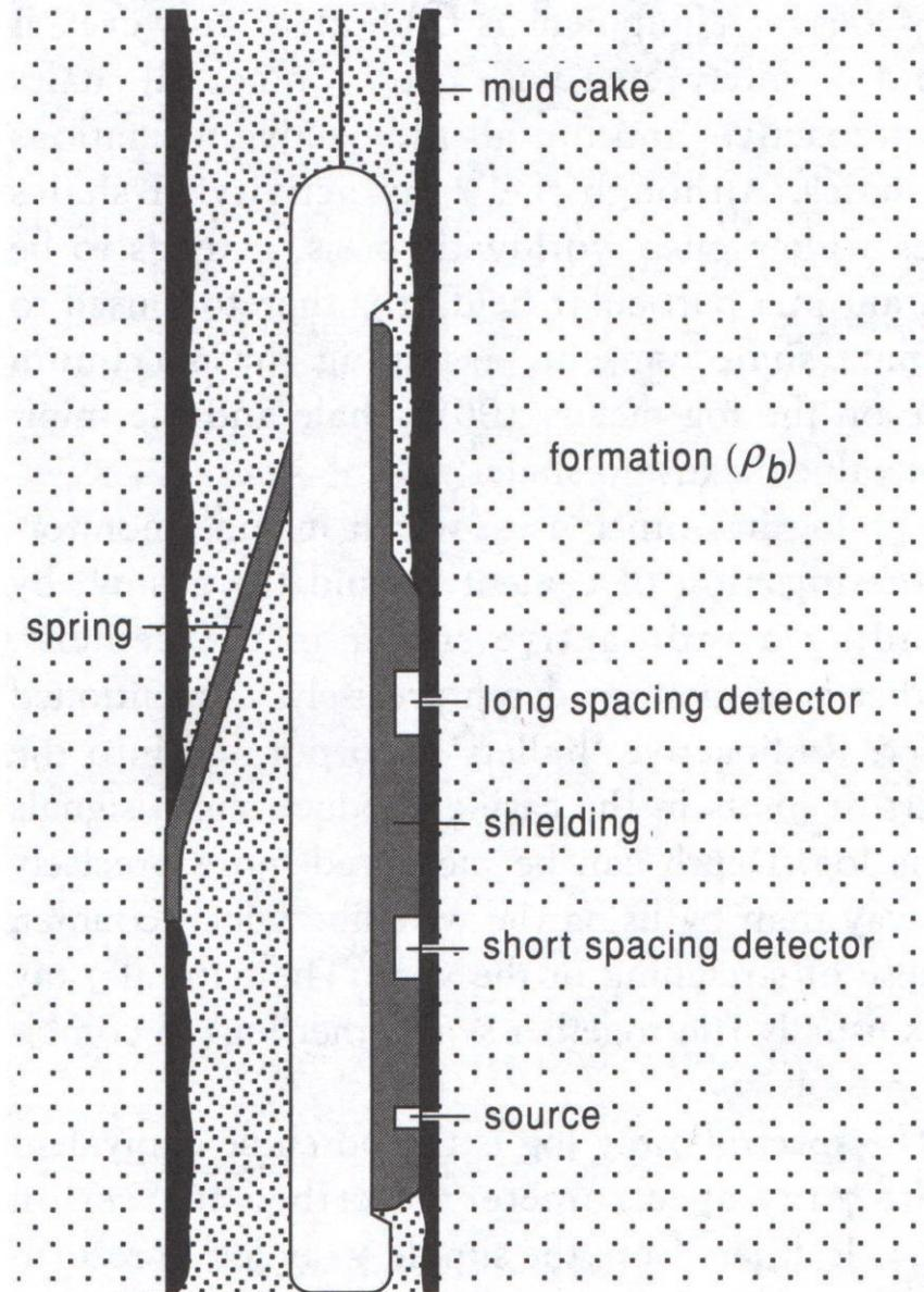
**Figure 18.11** The  $\gamma$ - $\gamma$ , or formation density, logger.
