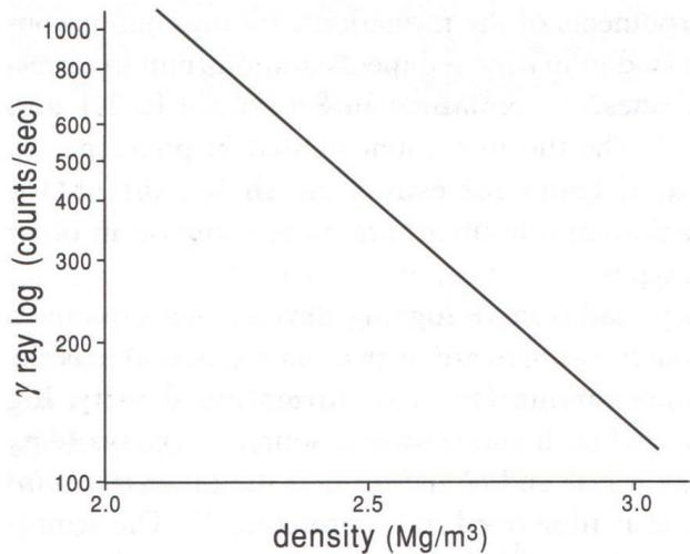
**Figure 18.12** Relation between density logger count and density.
