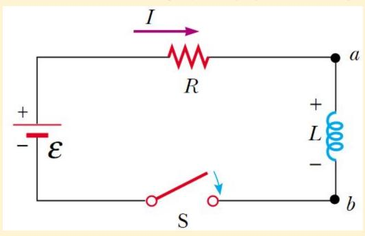
An inductor in a circuit opposes changes in the current in that circuit:
