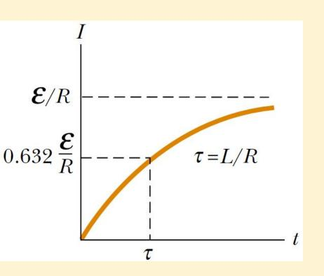
The time constant  $\tau$  is the time interval required for I to reach 0.632 (1-e<sup>-1</sup>) of its maximum value.
