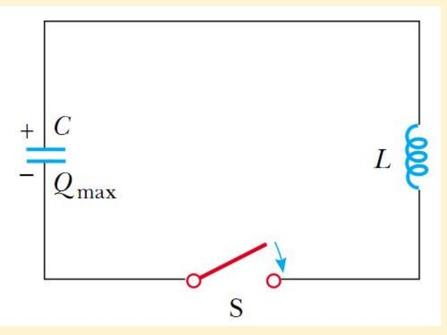
If the capacitor is initially charged and the switch is then closed, we find that both the current in the circuit and the charge on the capacitor oscillate between maximum positive and negative values.
