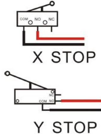
PS: For auto level 3D printer, there only 2pcs limit switches , one for X-axis and one for Y-axis, the Position sensor is for Z stop and auto leveling .
