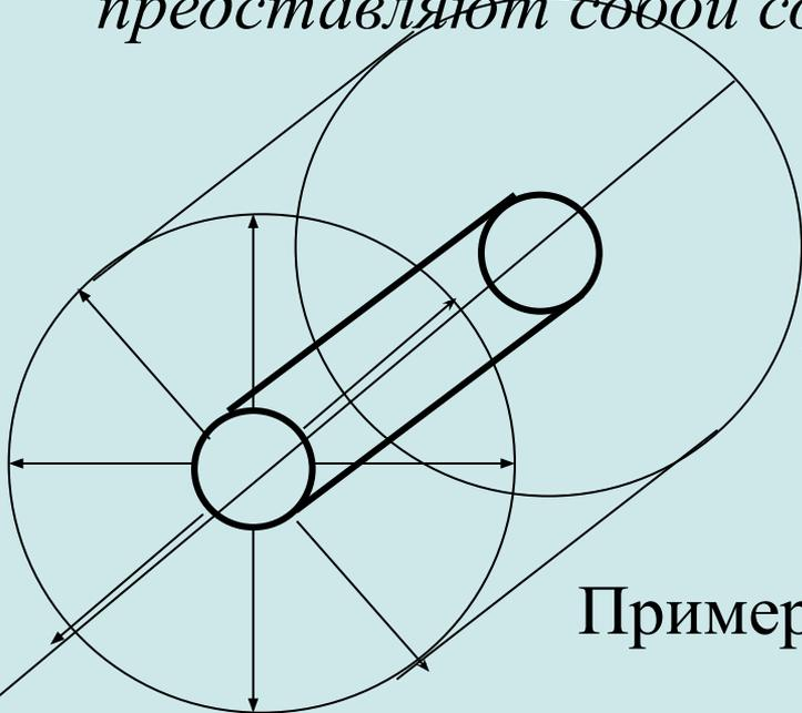
$$R_{rc} = \rho \frac{\ln \frac{r_2}{r_1}}{2\pi \cdot l}$$
