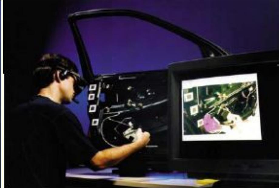
**Augmented Reality can be used for training as well as for assembly purpose**
