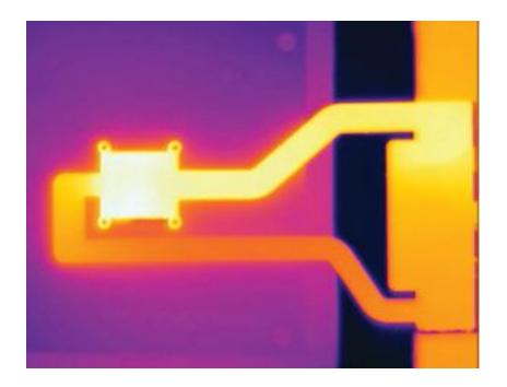
Fujitsu's superslim refrigerator is designed to suck heat out of a smartphone.
