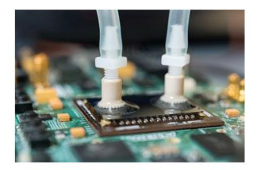
Water flows through microchannels on a chip.
