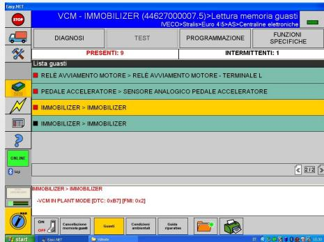
This fault DTC: B7 IMF: 02 indicates that the VCM is IN THE STATE IN WHICH IT IS NOT 'STILL ABLE TO GET THE STORAGE OF 2 KEYS.
