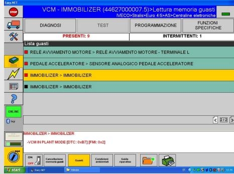
This fault DTC: B7 FMI: 02 indicates that the VCM is IN THE STATE IN WHICH IT IS NOT 'STILL ABLE TO LEARNING THE STORAGE OF 2 KEYS.
