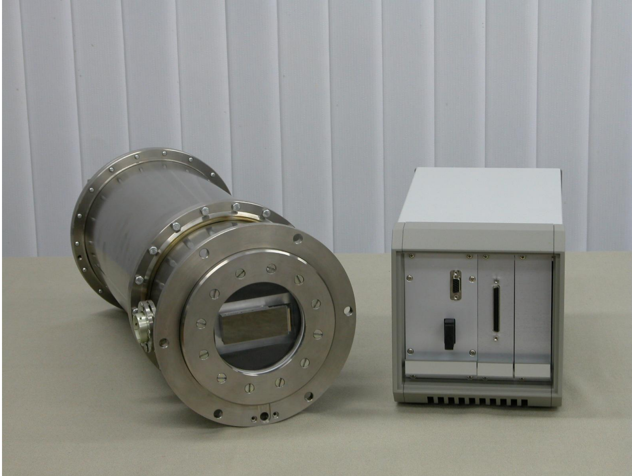
Camera 2K x 4.5k and controller (without power supply)
