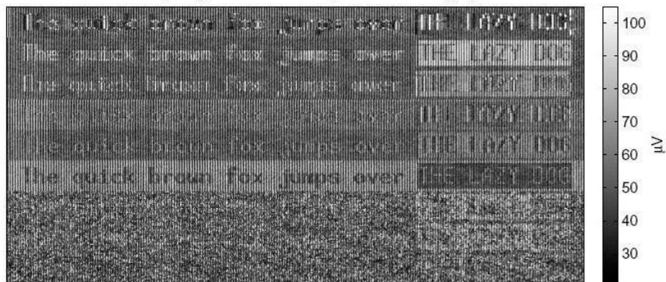
285 MHz center frequency, 50 MHz bandwidth, 16 frames averaged, 3 m distance
