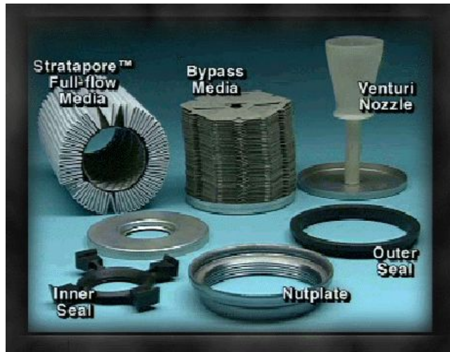
LF 9000 oil filter components
