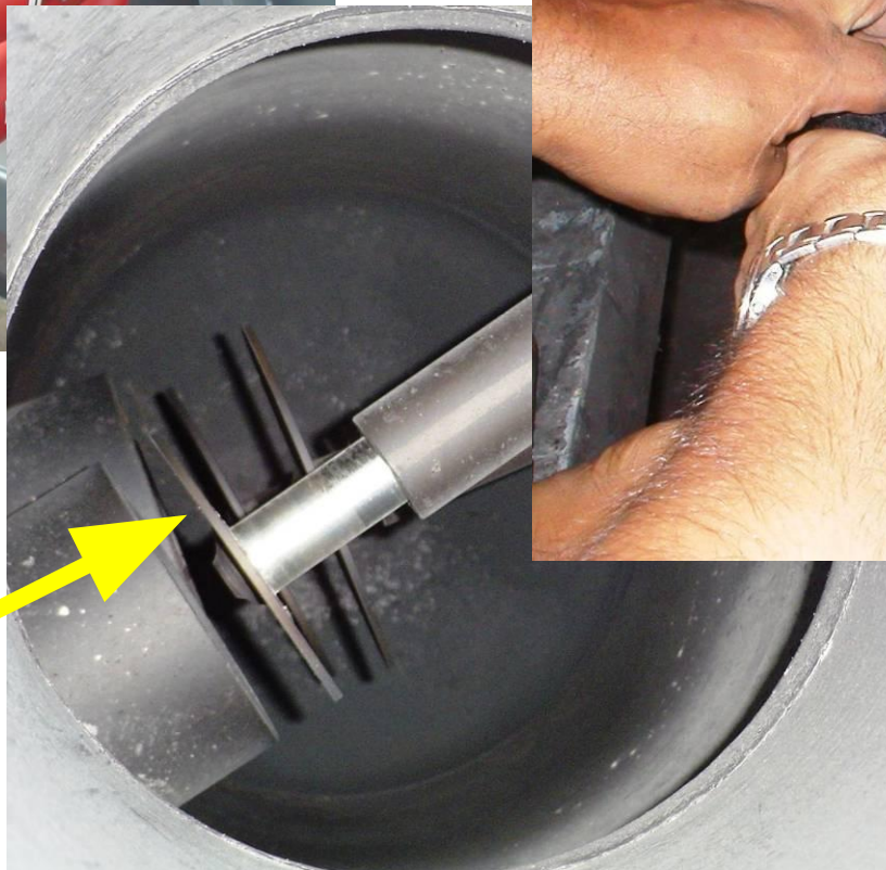
Anemometer for air speed measuring
