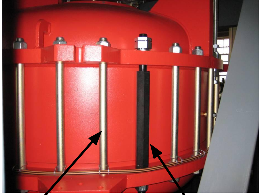
adjusting screws (black) washers should be moveable by hand
