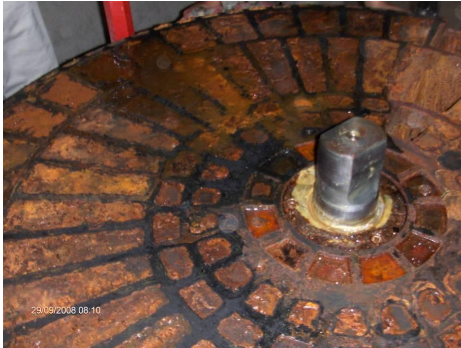
rusty bottom sealing plate
