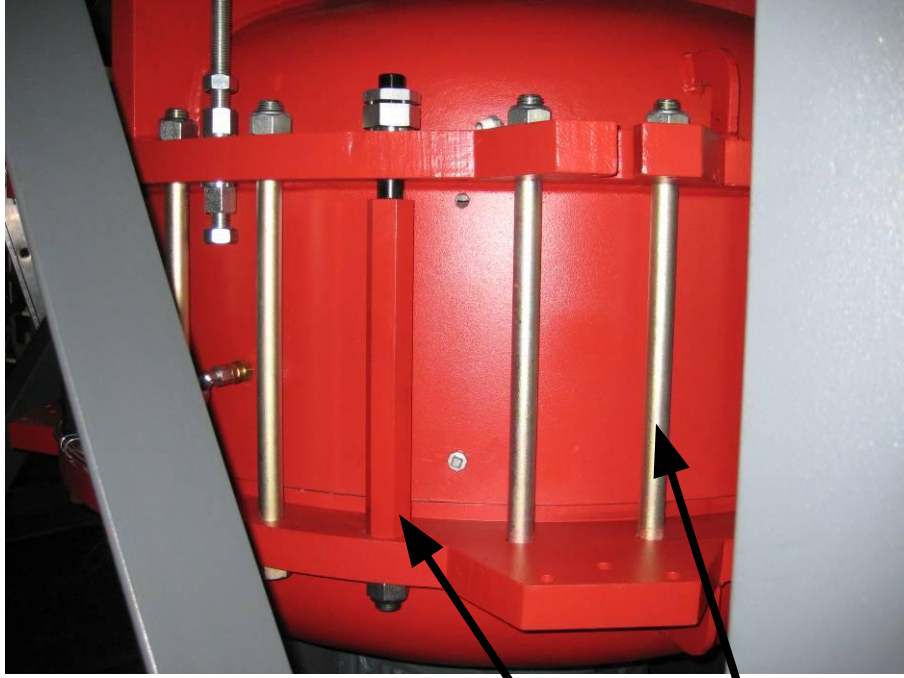
setting screws (red) for correct gap adjustment 0,25 mm
