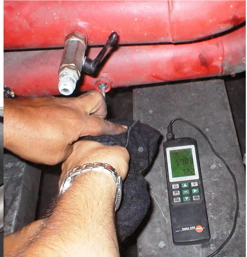
Anemometer for air speed measuring
