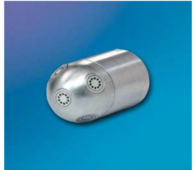
A 6.35 mm, 5-hole, fast-response probe. The probe has five Kulite XCS-062 transducers
