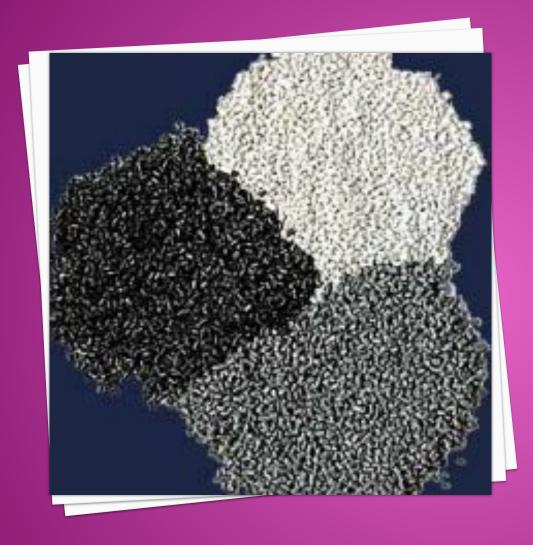
UNLIKE METALS, THE **PROPERTIES OF MOST PLASTICS VARY CONSIDERABLY WITHIN NORMAL OPERATING** TEMPERATURES. A PARTICULAR ACRYLONITRILE **BUTADIENE STYRENE (ABS)** WHOSE TENSILE STRENGTH IS 5500 LB/IN2 AT ROOM **TEMPERATURE CAN DROP TO** 2800 LB/IN2 AT 125°F. OTHER PROPERTIES ARE ALSO AFFECTED. FOR EXAMPLE, **BRITTLENESS INCREASES AS** THE TEMPERATURE DROPS, ETC.
