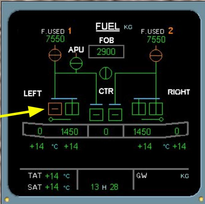
The left tank pump 1 is off, (cross-line amber).
