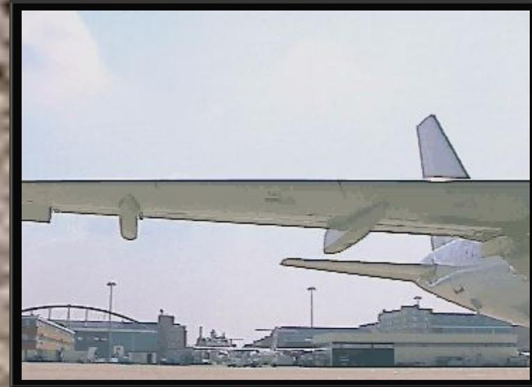
**A single refueling point is installed under the right wing. You should check that the refuel coupling door is closed.**
