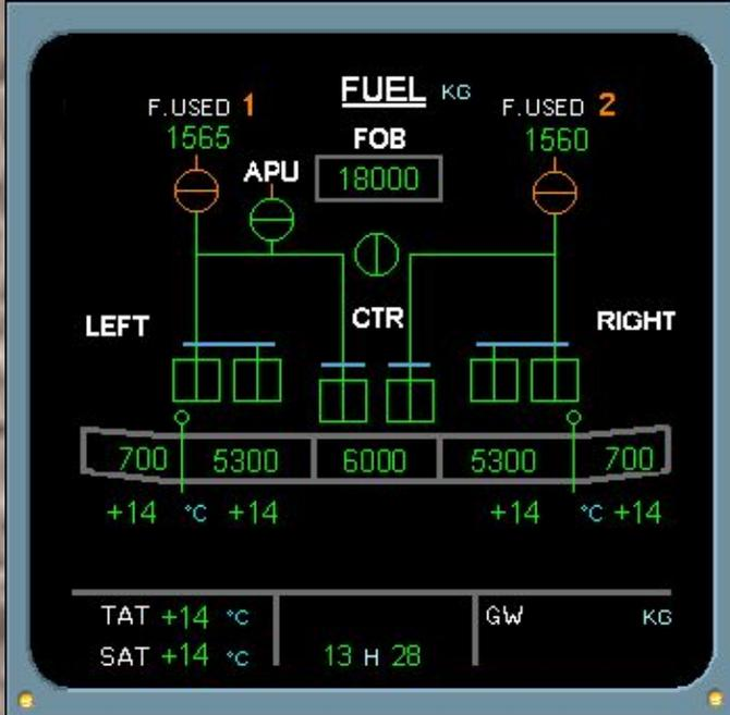
A few minutes later you observe that the refueling message on the E/WD has disappeared, indicating that refueling is complete and the refueling control panel door is closed.
