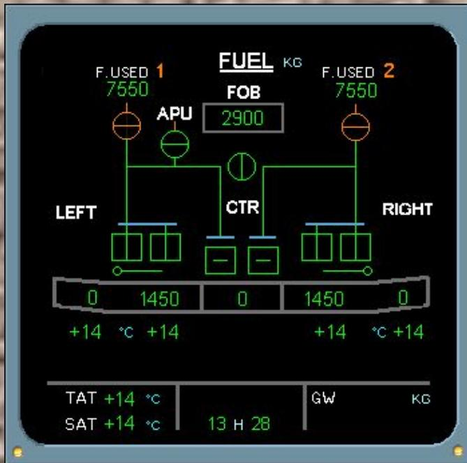
After the engines are shutdown, the fuel pumps are switched off.
