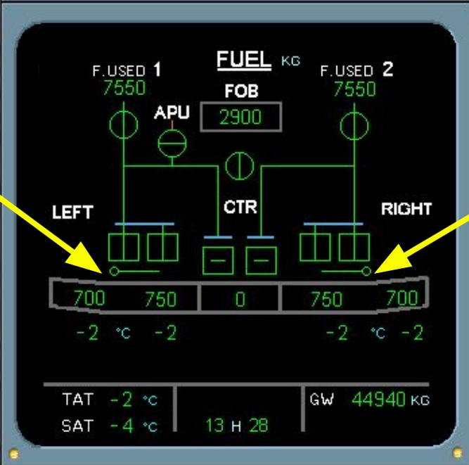
When either inner tank reaches a low level limit, both transfer valves open automatically transferring fuel from the outer to the inner tanks.
