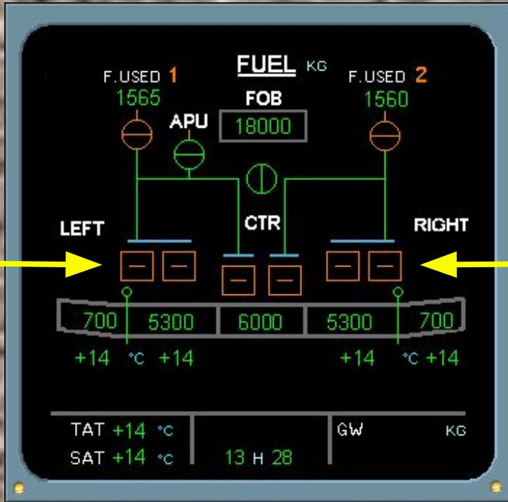
With the pumps in the OFF position, observe the symbology on the ECAM. The pumps are cross-line amber.
