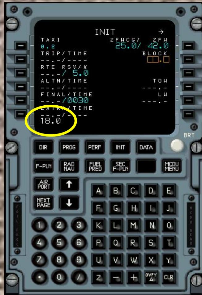
We have typed the fuel weight in the scratch pad for you.
