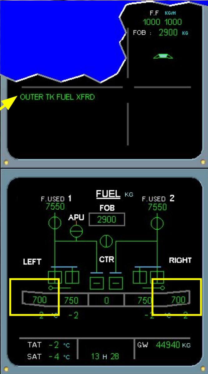
After at least one transfer valve is open, the message OUTER TK FUEL XFRD is displayed on the E/WD.
