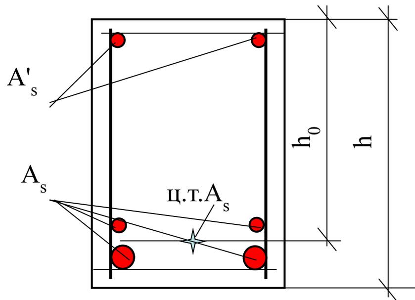
$$M_{пр} = R_s A_s Z_b \quad M_{оп} = R_s A_s Z_{b1}$$
