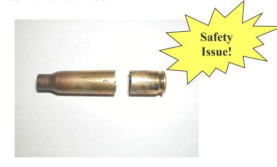
Condition requires the bolt to be replaced. Occurs at or before 6,000 rounds under extreme dust test conditions.
