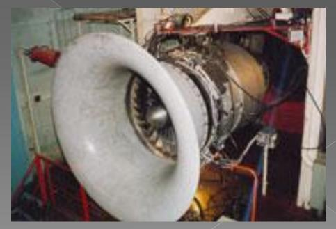
The D-36 engine has proven to be good in operation and reliable and has a very long designed and overhaul life
