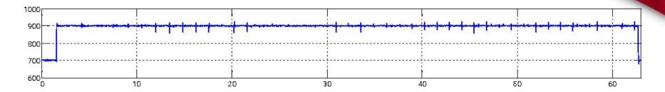
This is the beginning of the SCR efficiency test. The efficiency is determined for each of the three defined ANR's (.5, 1.0,2.0)
