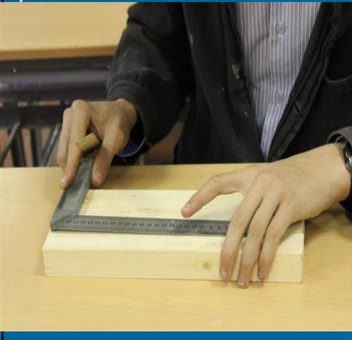
A close-up photograph showing a person's hands working on a light-colored wooden board. The person is using a square tool to draw a line on the wood, with a pencil held in their right hand. The board is resting on a wooden workbench. | Линейка, угольник                         |
