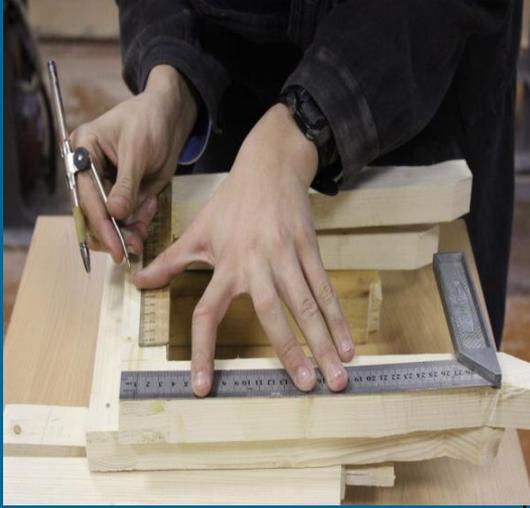
A close-up photograph showing a person's hands working on a wooden board. The person is using a compass to draw a circle on the wood. A ruler is placed horizontally across the board to measure the distance from the edge to the center of the circle. The person is wearing a dark jacket and a watch. | Линейка,<br>карандаш,<br>угольник, циркуль |
