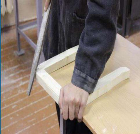
A close-up photograph showing a person's hands using a hand plane to smooth a light-colored wooden surface. The person is wearing a dark jacket. The background shows a workshop setting with a wooden floor and some equipment. | Рашпиль,<br>напильник,<br>наждачная<br>бумага |
