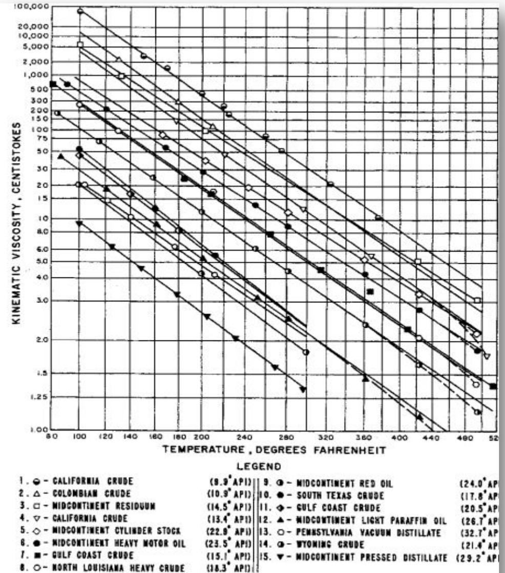
Fig. 8.1—Typical viscosity/temperature relationship for a heavy oil.<sup>6</sup>
