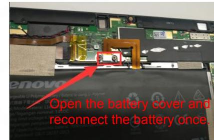
Open the battery cover and reconnect the battery once.
