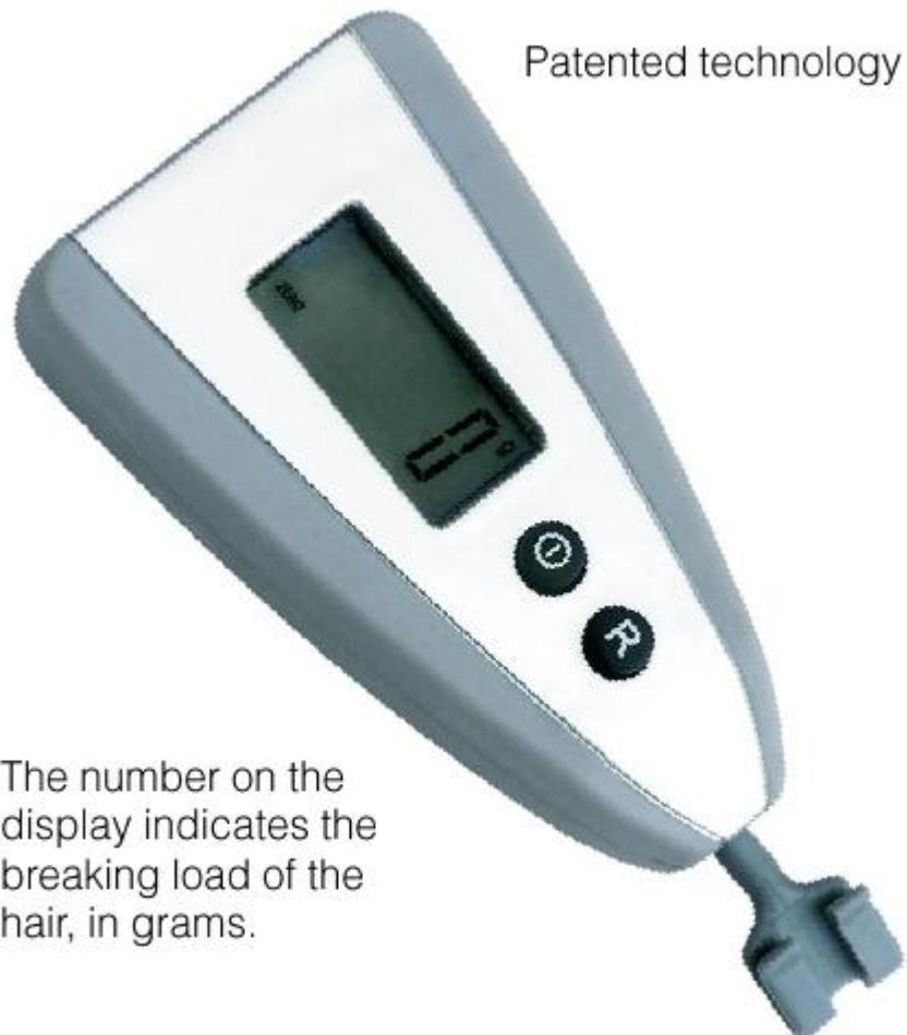
The number on the display indicates the breaking load of the hair, in grams.
