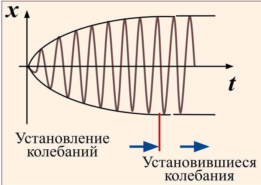
$$\frac{d^2 x}{dt^2} + 2\beta \frac{dx}{dt} + \omega_0^2 x = \frac{F_0}{m} \cos \omega t$$
