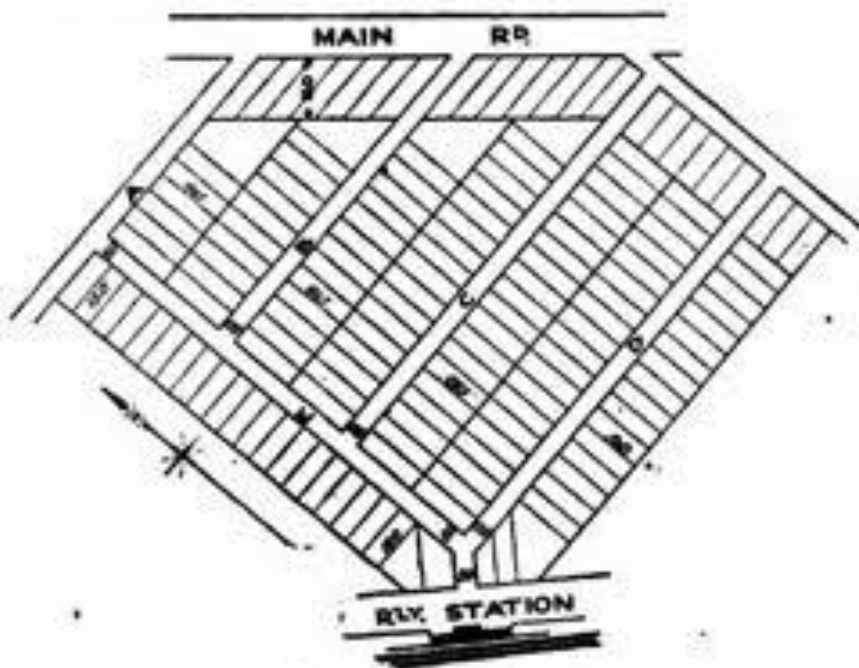
Checker-board Subdivision (old style)—150 lots, each with 30% frontage and depths of 150% to 170%.
