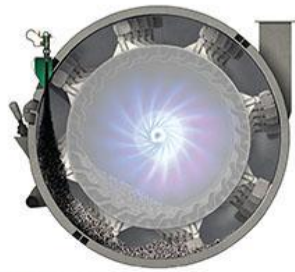
Liquid Asphalt Liquid asphalt is injected into the mixing chamber through the AC inlet or optional Warm Mix System
