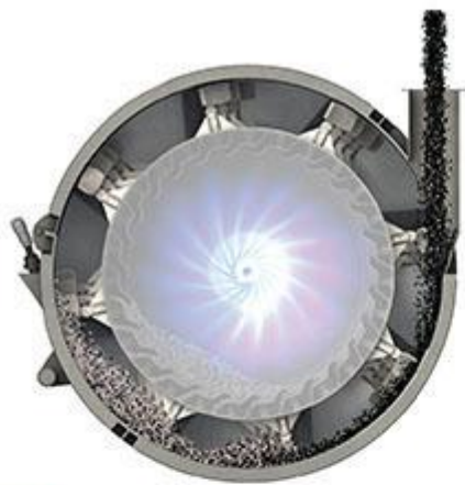
RAP (Recycled Asphalt Pavement) RAP material is added to the aggregate in the mixing chamber
