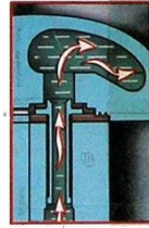
WATER TRANSFER FROM CYLINDER SLEEVE TO COVER
