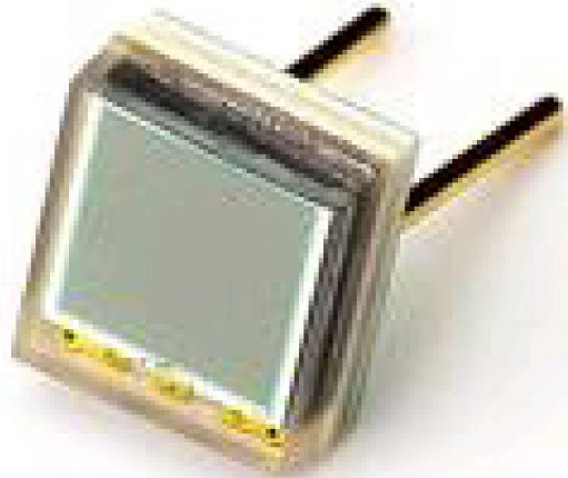
SiPM Ketek (PM3350), Gain~ 10E^6 , 50um/cell
