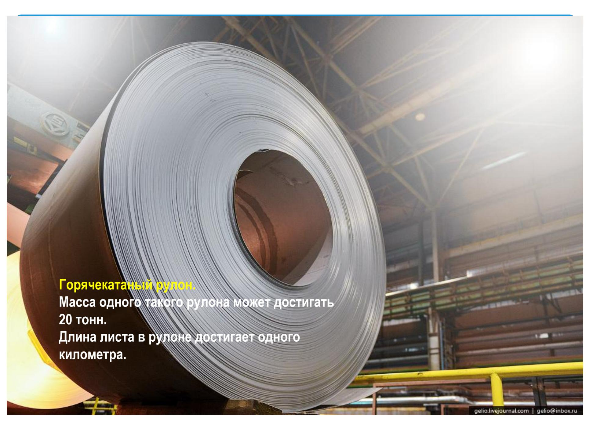
A large roll of hot-rolled steel is shown in a factory setting. The roll is massive, with a central hole, and is surrounded by industrial equipment and structural beams. The lighting is bright, highlighting the metallic surface of the steel.
