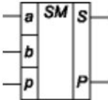
$$\left. \begin{aligned} S &= \bar{a}\bar{b}p + \bar{a}b\bar{p} + a\bar{b}\bar{p} + abp \\ P &= \bar{a}bp + a\bar{b}p + ab\bar{p} + abp \end{aligned} \right\}$$
