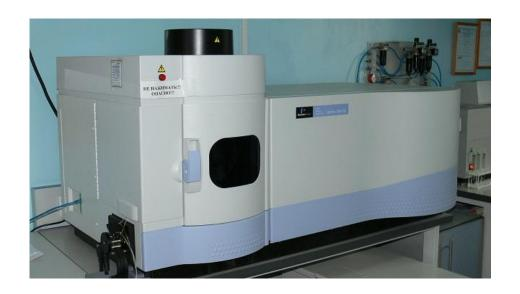
An atomic emission spectrometer is a highly sensitive device designed for the rapid determination of the elemental composition of a substance, recording radiation spectra in the range of 200-1000 nm.
