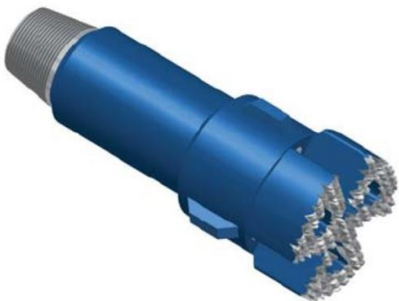
Fig.8. Junk mill. A slight concavity to the face of the mill helps to center the junk beneath the cutting surface so it can be ground into smaller pieces.
