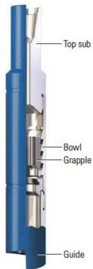
Fig.11. Overshot. The overshot is divided into three segments. The top sub connects the overshot to the workstring. The bowl has a tapered helical design to accommodate a grapple, which holds the fish in place. The guide helps position the overshot onto the fish.
