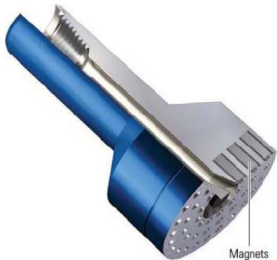
Fig.7. Junk magnet. This type of magnet is used to retrieve small pieces of ferrous material from the hole. Some junk magnets have circulating ports that enable cuttings to be washed away from the junk.
