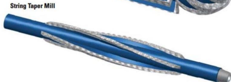
Fig.9. Downhole milling tools. Mills come in a variety of sizes and configurations. The taper mill ( top ) is designed for milling through tight spots and cleaning out collapsed or deformed tubulars. A pilot mill ( center ) may be employed to mill sections of tubular junk or to dress casing prior to installing a casing patch. The larger milling blades are guided by the small central pilot at the front of the tool. The string taper mill ( bottom ) may be used for cleaning out damaged tubulars and is also recommended for removing keyseats in open hole. Tapering at the top and the bottom of this mill allows it to ream in both directions.
