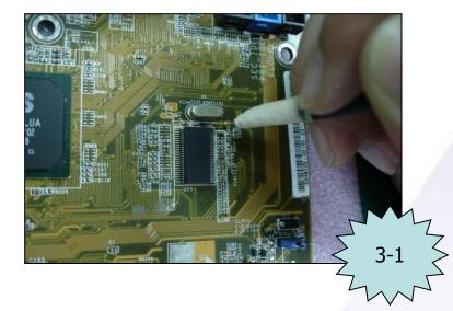
Use Oscilloscope to measure Clock X'TAL 14.318Mhz is ok.
