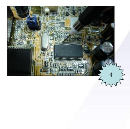
Use Oscilloscope to measure every individual CLK signal. If find error please trace the circuit to find it's connection.
