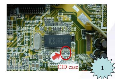
Visual Inspection to check Clock Generator and related small components are not damaged.
