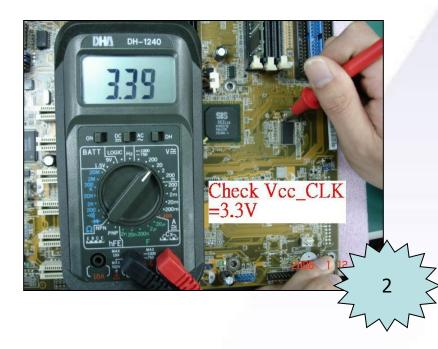
Use Multi-Meter or Oscilloscope to measure Clock voltage 3.3V is ok.
