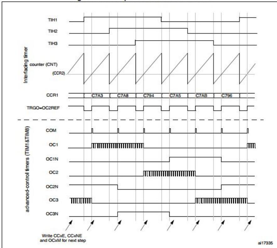
Figure 93. Example of counter operation in encoder interface mode.
