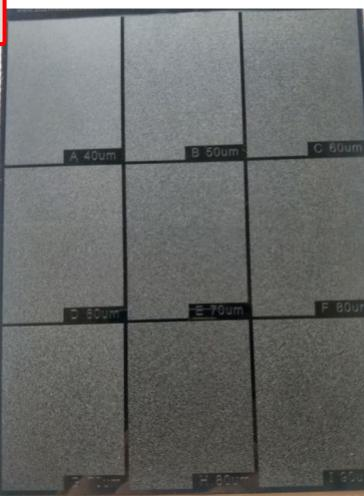
There is line around the top surface. It is recommended that the surface treatment of the product be changed from VDI24 to I90UM. Will lighten traces of the line.
