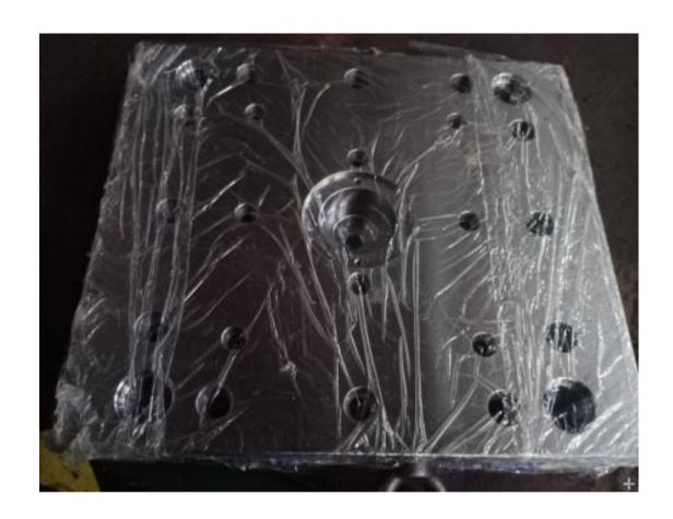
The template on the mold is very thin and deformed before, and the product is prone to burrs. We have replaced new template. Please know.
