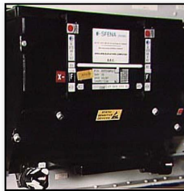
Spoiler and Elevator Computer (SEC)
