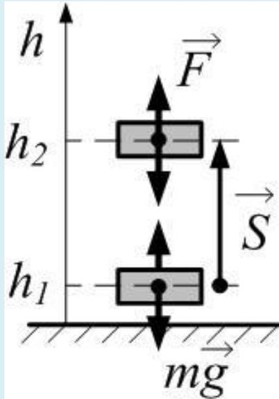
$$\begin{aligned}\Delta W &= W_2 - W_1 = A_{\text{внешн.сил}} = \int_1^2 \vec{F} \cdot d\vec{S} = \int_1^2 F \cdot dS = \\ &= F \int_1^2 dS = mg \cdot \int_{h_1}^{h_2} dh = mg \cdot (h_2 - h_1)\end{aligned}$$
