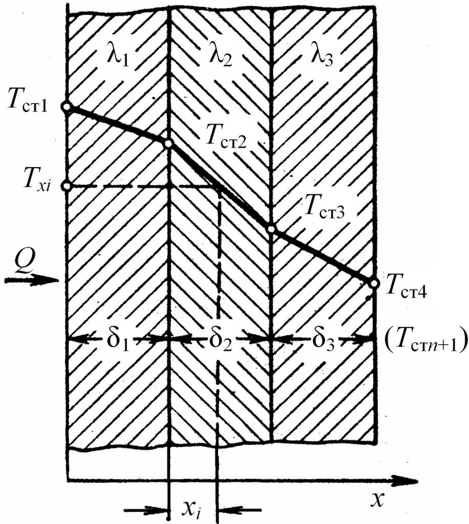
$$\left\{ \begin{aligned} \bar{q} &= \frac{\lambda_1}{\delta_1} (T_{cm1} - T_{cm2}) \\ \bar{q} &= \frac{\lambda_2}{\delta_2} (T_{cm2} - T_{cm3}) \\ &\dots \\ \bar{q} &= \frac{\lambda_n}{\delta_n} (T_{cmn} - T_{cm(n+1)}) \end{aligned} \right.$$
