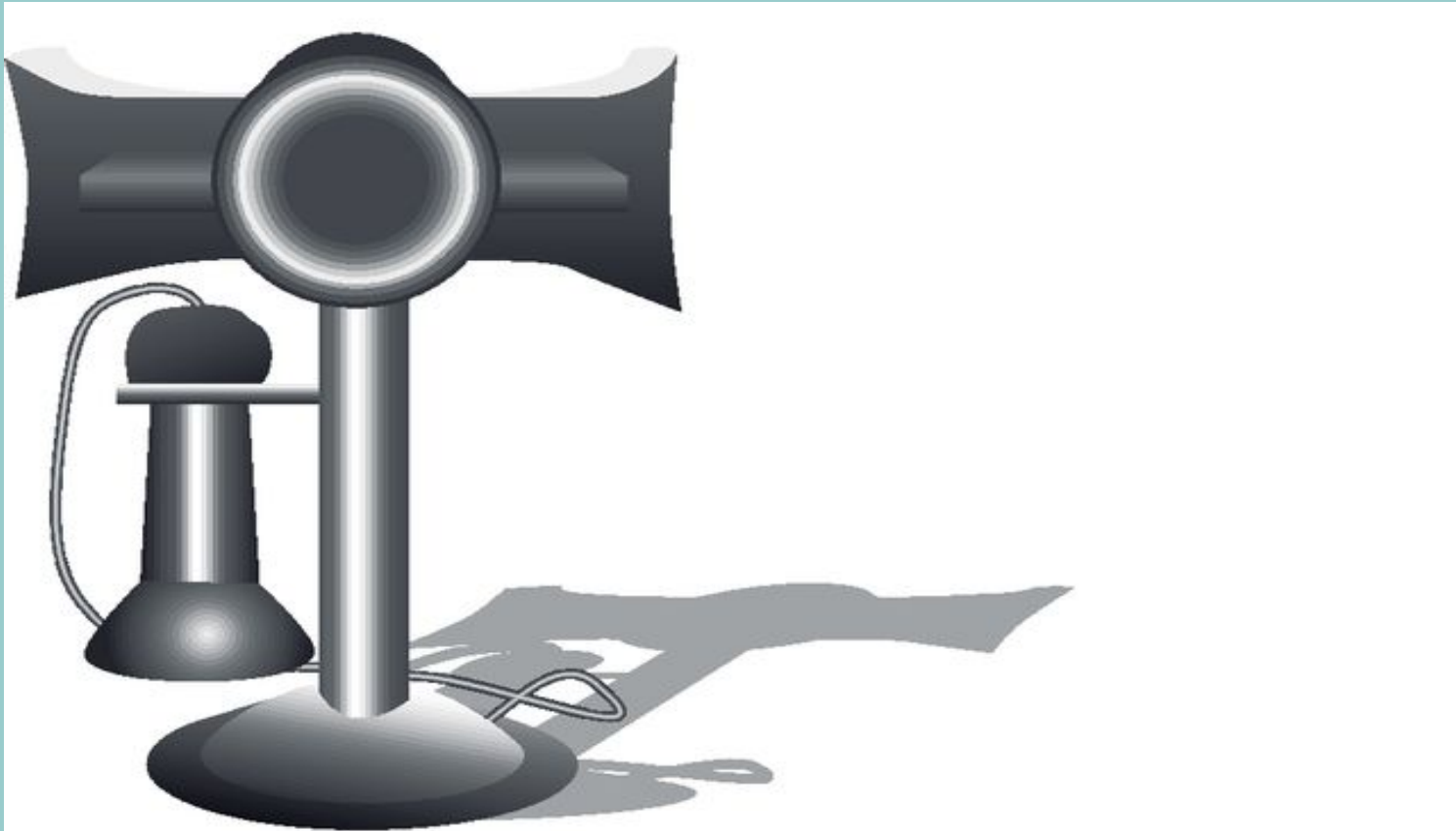
Figure 3-10 The Hush-a-phone telephone attachment
