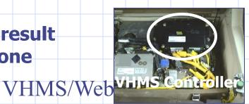
Record data into VHMS controller automatically
