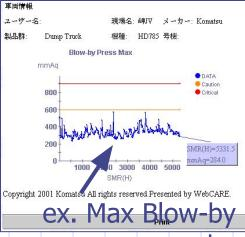
pressure can be found condition of internal parts wear
