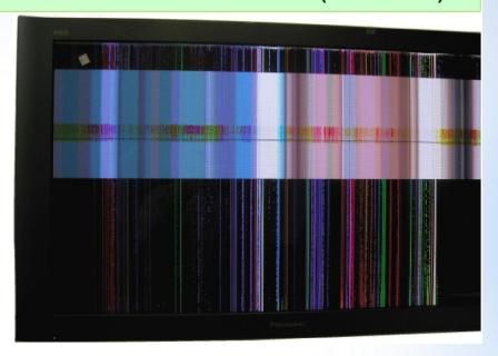
Disconnecting the SU board yields a good picture at the bottom half of the screen and a completely black area in the upper half of the screen.
