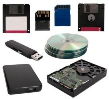
Storage hardware consists of the following elements: Hard disk (HDD), floppy disk and CD - ROM.
