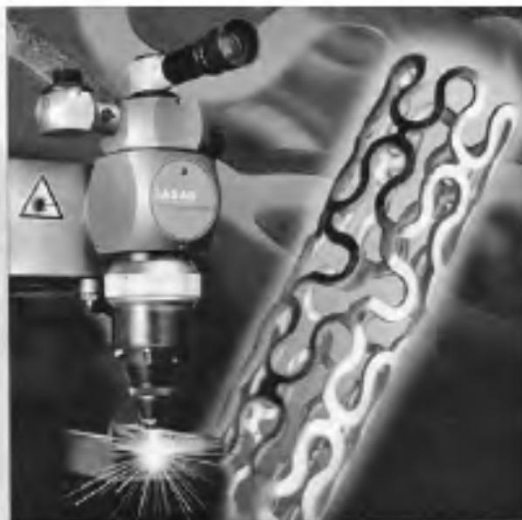
Pulsed YAG Laser: For fine cutting and welding
