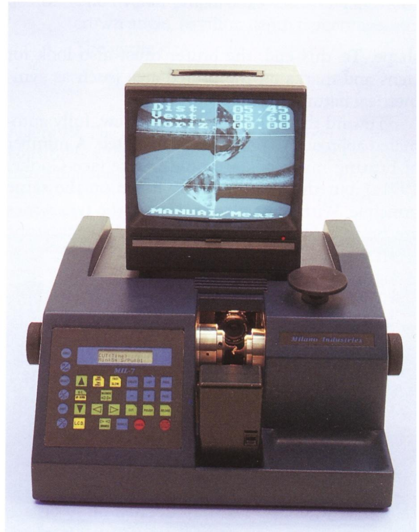
Figure 16. In this photo of an automated bruting machine built by Milano Industries in Israel, two diamonds are mounted for bruting to create a girdle surface on each by mutual abrasion. By viewing the screen, the operator can correctly position each stone and then monitor the progress of the bruting process. Photo courtesy of Milano Industries.
