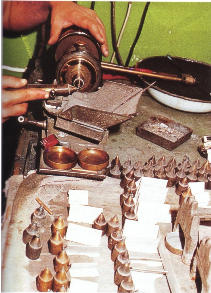
Figure 15. With a manual bruting machine, the diamond is glued to a dop that is set in the machine. In his hand, the bruter holds a stick with another dop to which a diamond has been glued. As the diamond in the machine is rotated, the other diamond is bruting it.
