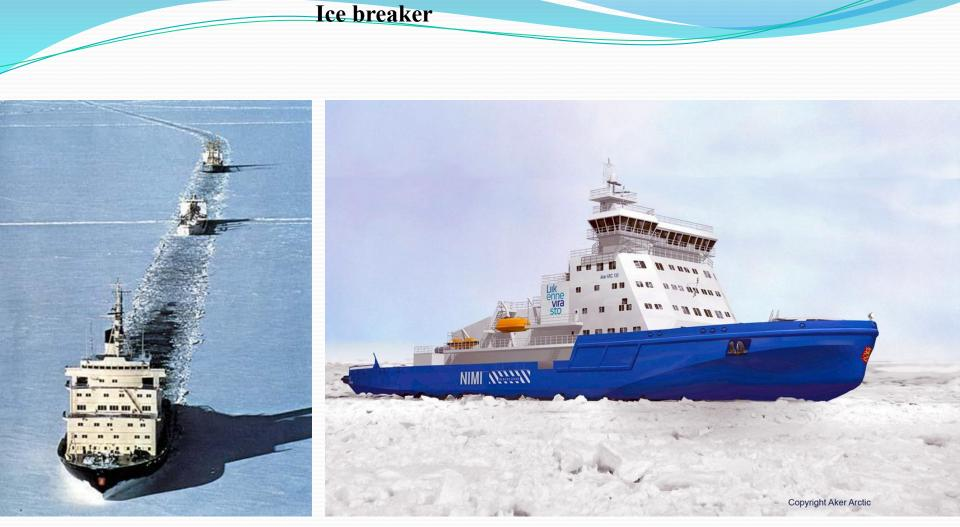
A self-propelled specialized vessel designed for various types of icebreaking operations in order to maintain navigation in freezing basins.
