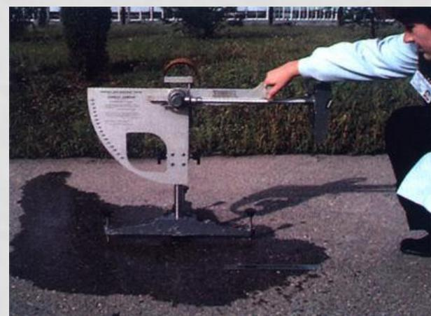
*Portable Skid Resistance Tester (SRT)*
